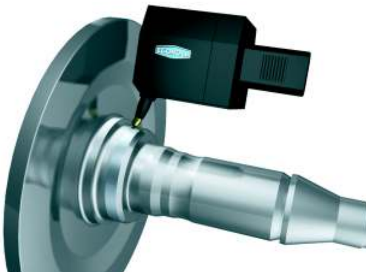
Deep rolling the fillet radius of an axle shaft to increase fatigue strength.
