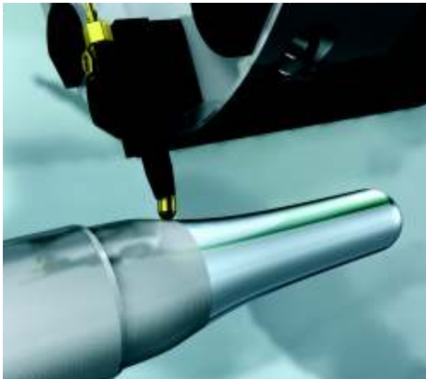
Machining a hard, contoured mandrel with an HG6 tool eliminates manual polishing.
